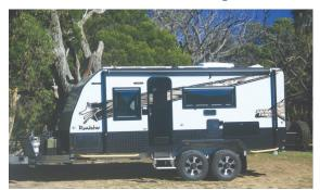
For example this Roadstar Caravan can carry a payload of 720kg. The ATM is 3500kg.
