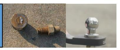
When I first started caravanning I was told that I should replace the tow ball about every two years because they do break, usually at the top of the thread, see the picture above. You can then carry the old one and use it as a replacement if you break one out in the middle of Australia. It is worth paying a few dollars more to buy a quality replacement.
